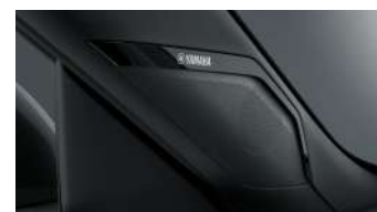
Front dome tweeter on A pillar
